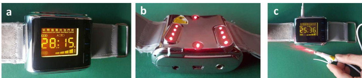
Fig. 1: Laser watch for laser acupuncture and laser blood irradiation (front (a), rear (b) and view with nasal adapter (c)).
